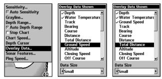
Overlay Data command on the Sonar Menu (left). Overlay Data Shown selection menu (center). In this example, we scrolled down the data list to highlight Ground Speed. It will be displayed in a small size. Data list with Total Distance selected (right).
